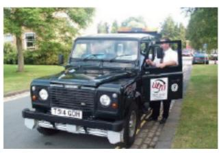
Digital maps and the survey routes are loaded onto the computer in the vehicle and the operator uses the 'touch sensitive screen' in the vehicle to select the first route to be surveyed. A map will appear on the screen showing the route, clearly defining the start and end points.
