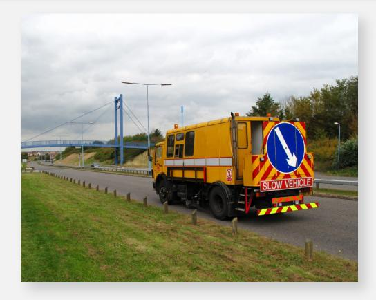
ed on a common reference frame resting on the road surface. The deflection beams and reference frame are stationary during the deflection measurement cycle and remain stationary until the maximum deflection has been recorded.
