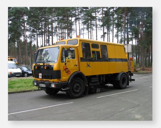
The reference frame is then pulled forward at twice the vehicle speed by a clutch and winch system to the initial position for the next measurement cycle. With the reference frame again at rest, the measurement cycle is repeated. This method of operation gives measurements of deflection in both wheelpaths at about 4 metre intervals. To travel between measurement sites, the Deflectograph measuring frame can now be picked up hydraulically, to ease the burden on operator and driver.
