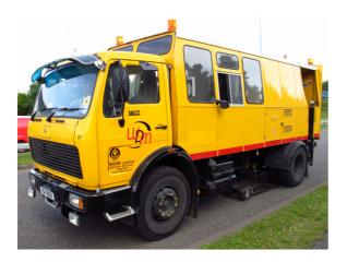
Deflectograph defines the backlog and long term budget requirements needed to maintain the structural integrity of the highway, It's used to measure the transient deflection of a road surface under the action of a rolling wheel at standard loading conditions. The measurements of deflection are used to assess the highway's structural condition and can be used to estimate the residual life of the networks, which is an essential input to asset management plans.
