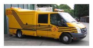
Road Assessment Vehicle (RAV). These vehicles provide measurements of the surface condition of a road, including cracking, to the SCANNER specification at normal road speed. The measurements monitor changes in the condition of networks and provide various key performance indicators helping clients prioritise maintenance.
