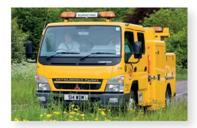
The SCRIM machine requires an operator and a driver. Skidding resistance data are recorded continuously by the SCRIM equipment and stored as an average for each 5, 10 and 20m section of road. The operator controls the survey and adds location markers to the data stream during the SCRIM machine survey.
