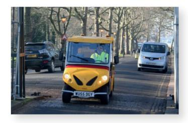
The Cyclopath has a forward facing camera capturing an image every five metres of forward travel during a survey. Images are 1280 x 768, 24bit RGB colour compressed Jpegs, saved as a Windows AVI file.
